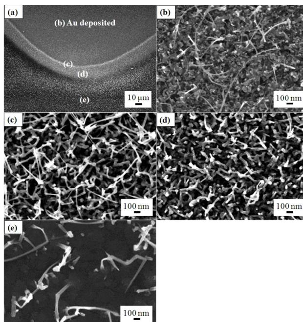
**Figure 1.** (a) FE-SEM images of  $\text{Ga}_2\text{O}_3$  nanowires grown on a 3 nm thick gold catalyst layer. Images (b)-(e) are magnified images of the areas indicated in image (a).
