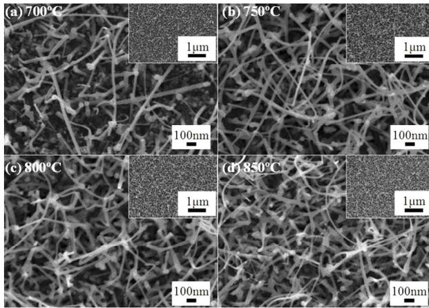
**Figure 3.** FE-SEM images of  $\text{Ga}_2\text{O}_3$  nanowires grown on 1 nm thick gold catalyst at growth temperatures of (a) 700°C; (b) 750°C; (c) 800°C; and (d) 850°C. The inset shows FE-SEM images scanned in wide range.
