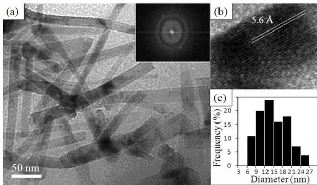
**Figure 4.** (a) TEM image of  $\text{Ga}_2\text{O}_3$  nanowires. Inset is SAED image; (b) Enlarged TEM image of a single  $\text{Ga}_2\text{O}_3$  nanowire; (c) Diameter distribution as obtained from TEM images.
