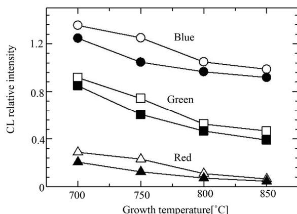
**Figure 6.** Growth temperature dependence of CL relative intensities for blue, green, and red emissions. Blank and filled symbols indicate as deposited and annealed  $\text{Ga}_2\text{O}_3$  nanowires, respectively.
