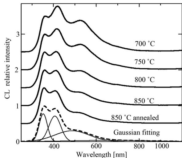
**Figure 5.** CL spectra measured for  $\text{Ga}_2\text{O}_3$  nanowires, as deposited at various temperatures in the range 700°C to 850°C, and nanowires annealed at 600°C after deposition at 850°C. The dotted line shows the fitting curve for four Gaussian curves (UV, blue, green, and red).
