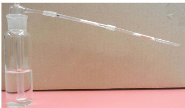
Figure 2. Experimental set up for speciation of Hg using ethylation based method.
