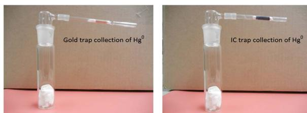
Figure 3. Experimental set up for emission of  $\text{Hg}^0$  from skin creams.
