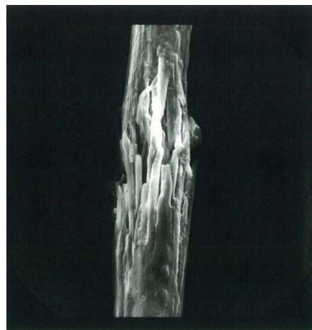
Figure 4. Damage as a result of hair relaxation. Insufficient rinsing is another possible reason besides damage due to combing or ironing after using solution 1.
