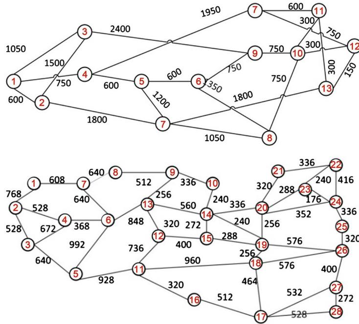
Figure 1. Topologies, (top) NSFNet network, (bottom) US Backbone network.
