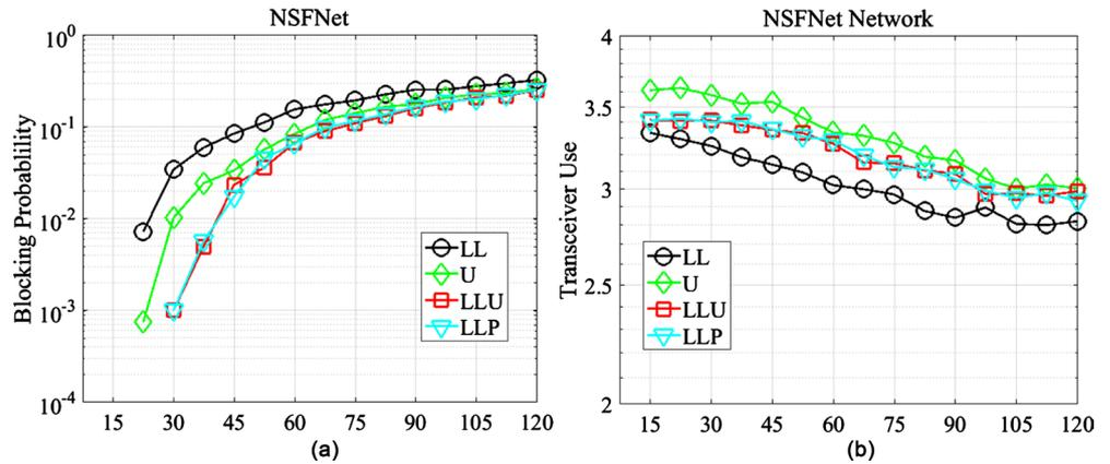
Figure 3. Performance (a) and resource utilization (b) of SPT using different cost metrics.
