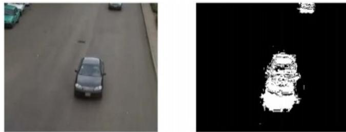
**Figure 2.** Moving object extraction through background subtraction.
