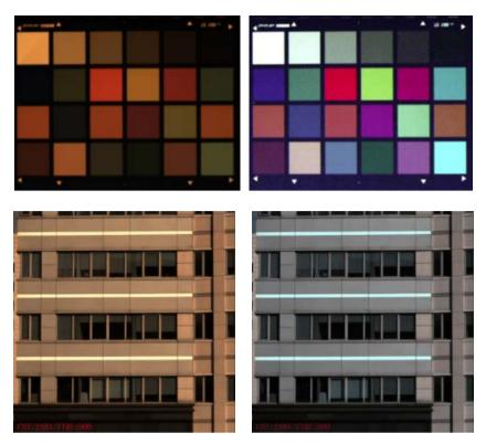
**Figure 7.** Color tranformation in lab and outdoor environment: (left) input image; (right) result.
