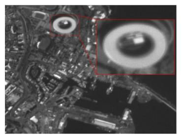
**Figure 2.** Raw image from OVS-1A covering Cape Town. Please zoom the electric version to see the mosaic phenomenon (Bayer format). Image is linearly stretched into [0-255] for visualization.
