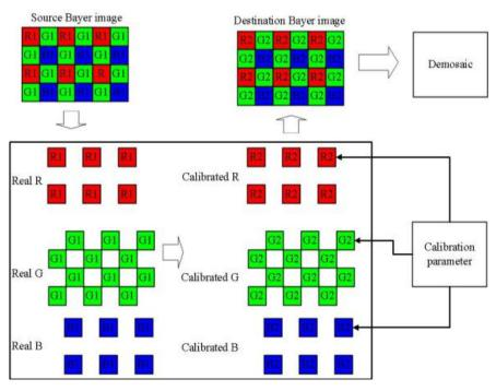
Figure 5. Pick out physically imaging pixel and reconstruct RGB image.
