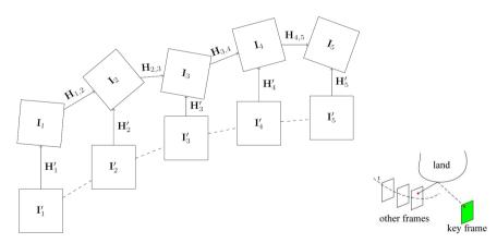
**Figure 9.** Illustration of the motion smoothing and imge registration.  $\{I_i\}_{i=1,2,\dots,n}$  is the initial image,  $\{H_{i,i+1}\}_{i=1,2,\dots,n}$  are the computed transformations.  $\{I'_i\}_{i=1,2,\dots,n}$  is the stabilized sequence and  $\{H'_i\}_{i=1,2,\dots,n}$  the stabilizing transformations [10].
