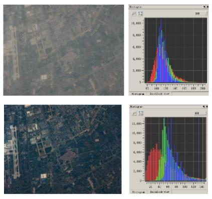
**Figure 8.** Radiometric calibration for Bayer video sequence (image is zoomed in for better analysis, covering Houston): (left) initial calibration (Bayer to RGB); (right) after no-uniformity correction from [7].
