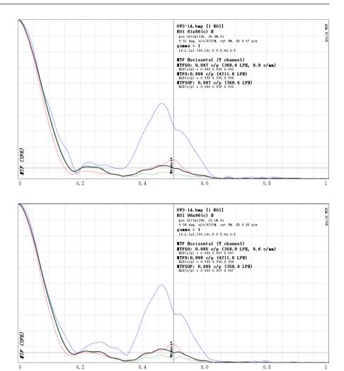
**Figure 11.** MTF curve of OVS-1A (above) and OVS-1B (bottom). Bayer video mode lowers the MTF value from classical 0.1@Nyquist frequence to 0.08 and the blue channel decreas too fast.
