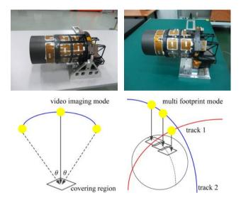
**Figure 1.** Camera in lab and Imaging mode: (Top left) OVS-1A; (Top right) OVS-1B; (Bottom left) video sequences; (Bottom right) multi footprint to get large region.
