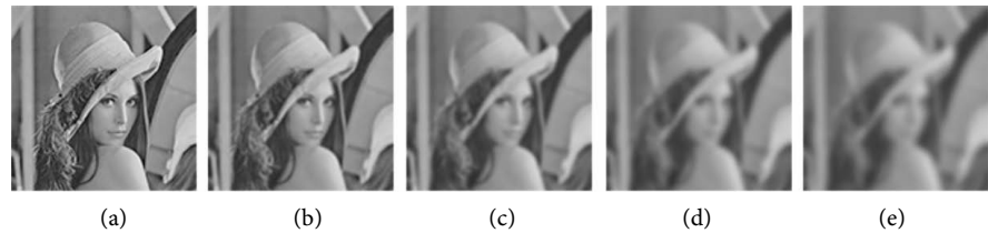
Figure 4. Initial and blurry images of Lena images, (a) Initial Lena image with D(f) = 1.0000 ; (b) Lena images blurred with a Gaussian radius of 2.5 with D(f) = 0.1117 , Lena images blurred with a Gaussian radius of 5 with D(f) = 0.0920 ; Lena images blurred with a Gaussian radius of 7.5 with D(f) = 0.0842 ; Lena images blurred with a Gaussian radius of 10 with D(f) = 0.0797 .
