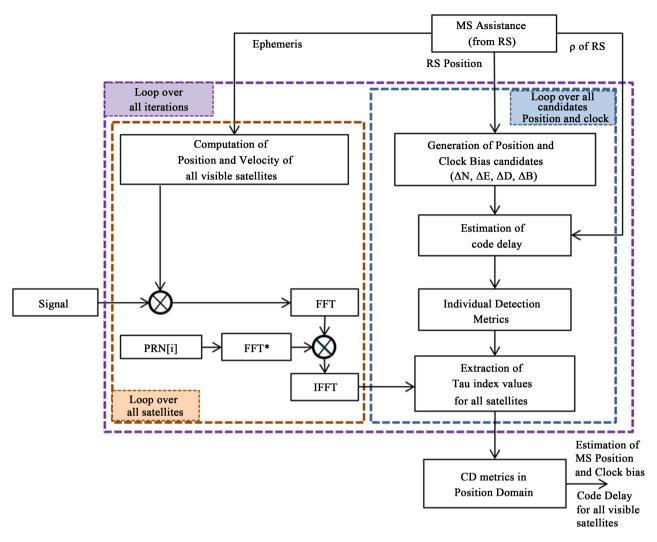
Figure 2. Block diagram of collective detection.
