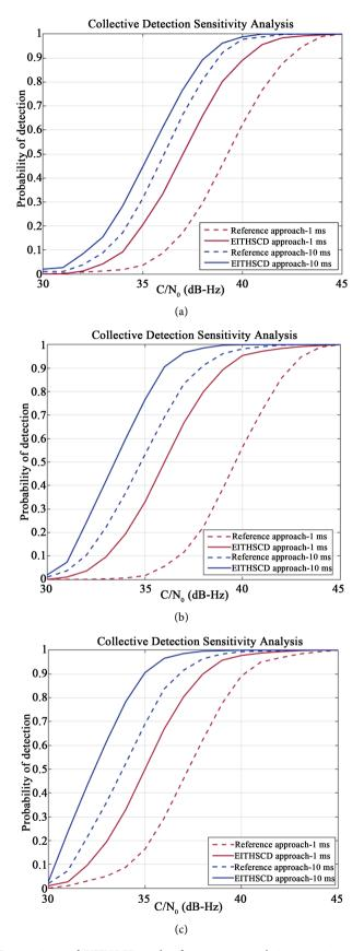
**Figure 4.** Comparison of EITHSCD and reference approach in sensitivity performance. (a) Scenario 1; (b) Scenario 2; (c) Scenario 3.
