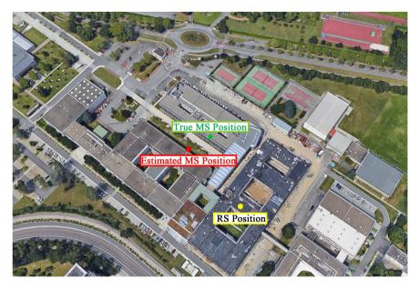
Figure 9. Position error obtained from EITHSCD algorithm.
