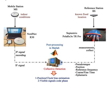
Figure 5. Setup of CD process and real signal acquisition (NordNav R30 as MS & Septentrio PolaRx3e as RS).
