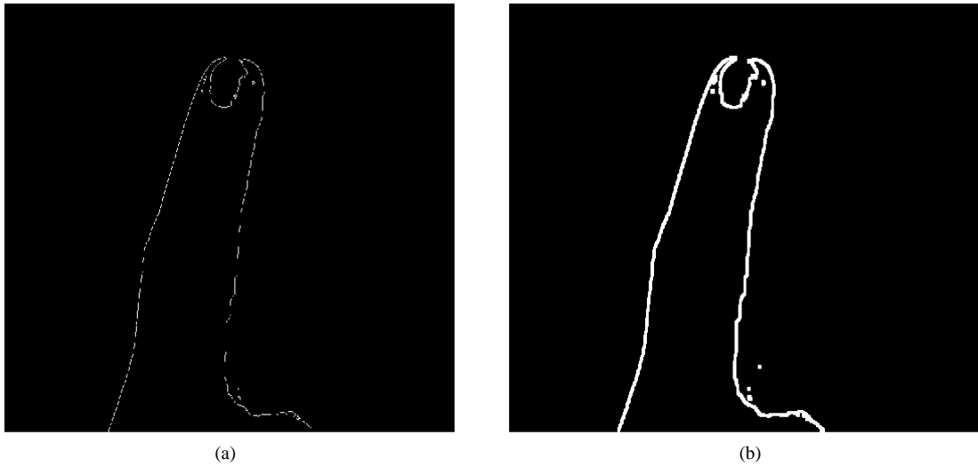
Figure 3. The results attained with (a) Edge Detection and (b) Edge Enhancement Schemes.
