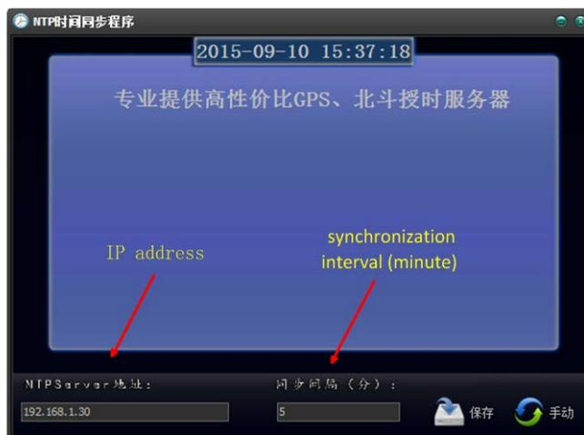
Figure 9. The client interface of NTP server.
