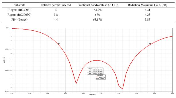
Table 1. Antenna bandwidths and gains with different substrates.
