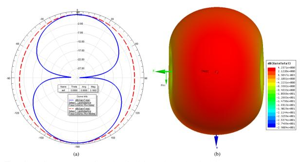
Figure 6. Radiation power pattern (a) in two dimensional view; (b) in three dimensional view.
