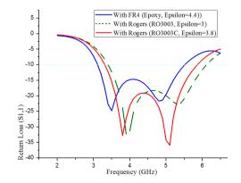
Figure 2. RL with different substrates.
