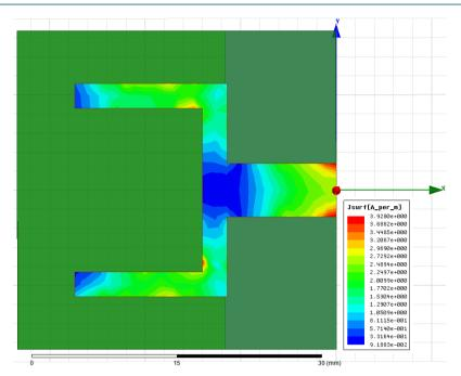
Figure 8. Magnitude surface current density.
