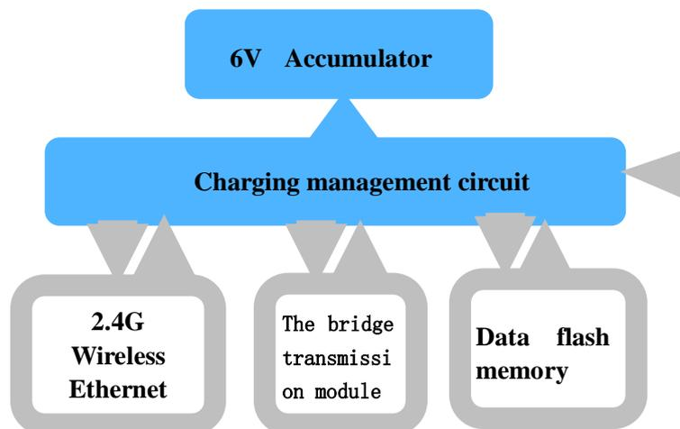
Figure 3. Hardware architecture of monitoring base station.
