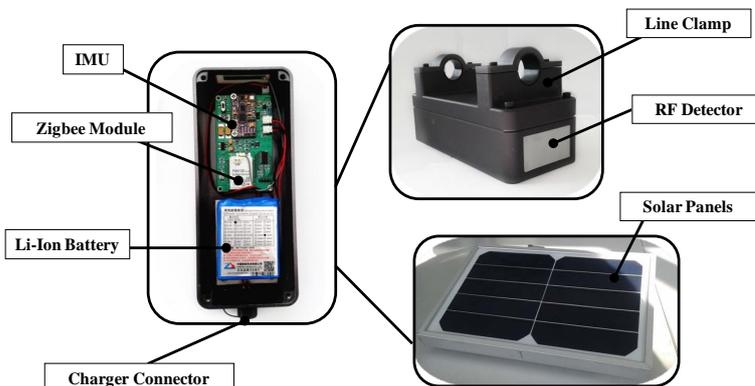
**Figure 2.** Hardware components of WIMU.
