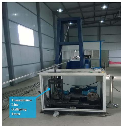
**Figure 5.** Galloping testing machine.
