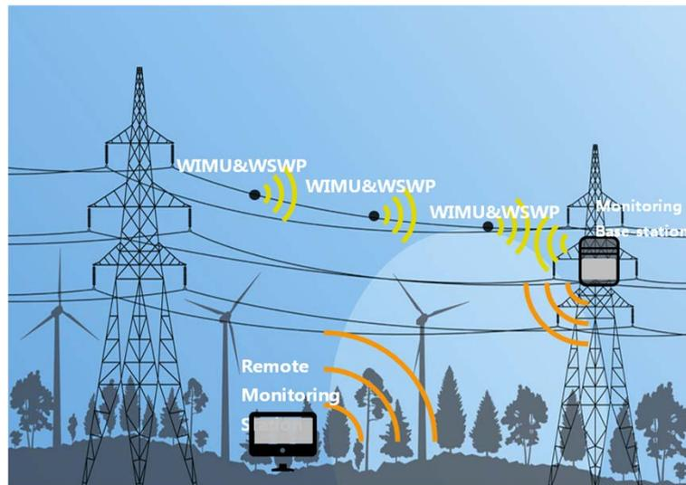
**Figure 1.** Schematic of WIMU-based galloping track online monitoring system for transmission lines.
