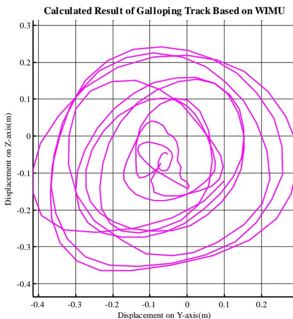
**Figure 8.** Reconstructed motion track in approximate circular motion case.
