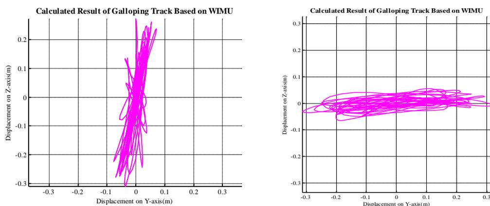
**Figure 7.** Reconstructed motion track: a) in vertical motion case; b) in horizontal motion case.
