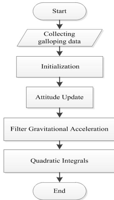
**Figure 4.** Algorithms for reconstructing galloping track of transmission lines.
