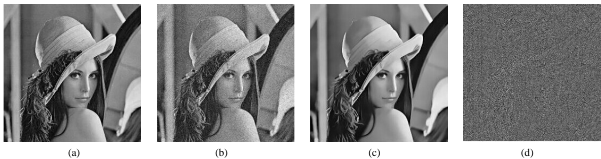
Figure 1. Recovered results via the original non-local means algorithm. (a) Original image; (b) Noisy image; (c) Filtered image; (d) Residuals.
