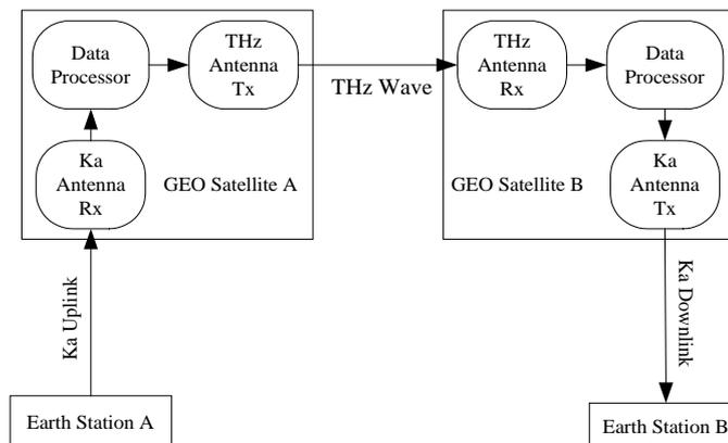
**Figure 2.** Block diagram of MODE 1 (GEO-GEO link).
