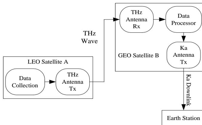
Figure 3. Block diagram of MODE 2 (LEO-GEO link).
