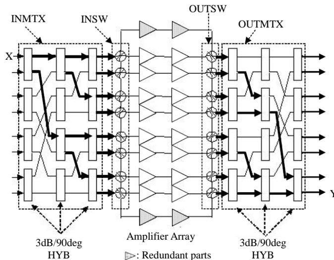
**Figure 6.** Block diagram of MPA.
