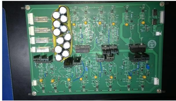
**Figure 5.** PCB board fabricated of designed circuit.
