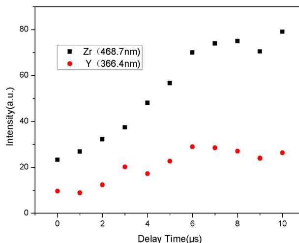
Figure 2. Intensity vs. gate delay time for the Y II 366.4nm and Zr I 468.7nm (#56).
