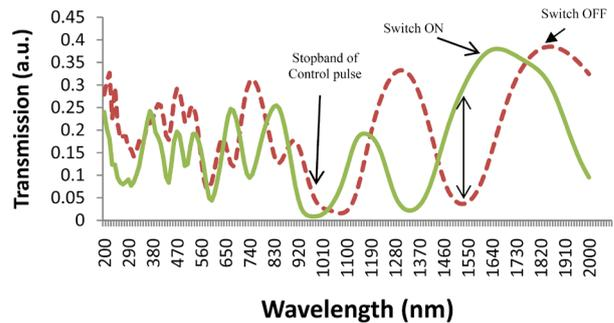
**Figure 5.** The overall transmission of the switch in OFF (dashed) and ON (solid) state.
