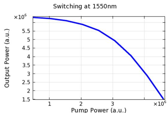
**Figure 7.** Dependence of Output power of the 1550 nm signal to power of the 1000 nm pump.
