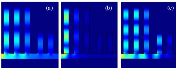
**Figure 4.** Intensity distribution of (a) 1550 nm at “on” state (b) 1550 nm at “off” state (c) 1000 nm as pump signal.
