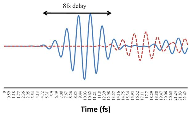
**Figure 6.** The temporal simulation of the switch shows a 8 fs delay in response.
