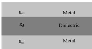
**Figure 1.** Schematic diagram of a metal-insulator-metal waveguide.
