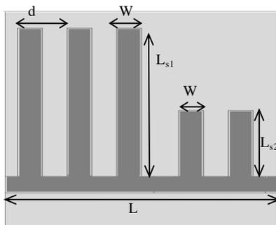
**Figure 3.** The proposed structure utilizing two stub filters based on MIM plasmonic waveguide.
