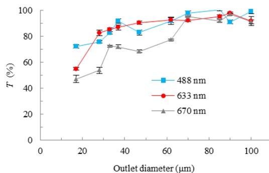
**Figure 4.** Transmittance of laser beam through the capillary of the 1.8 mm inlet diameter as a function of the outlet diameter with the optical lens.
