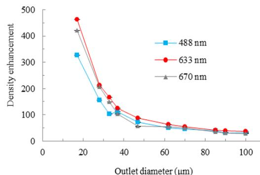
**Figure 7.** Density enhancement of the capillary for the 1.8 mm inlet diameter as a function of the outlet diameter without the optical lens.
