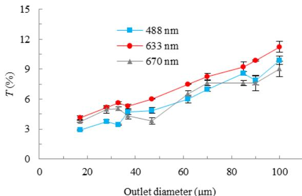
**Figure 2.** Transmittance of laser beam through the capillary of the 1.8 mm inlet diameter as a function of the outlet diameter without the optical lens.
