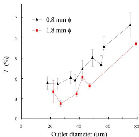
**Figure 5.** Comparison of transmittance through the capillary between the 1.8 mm and 0.8 mm inlet diameters at 633 nm.
