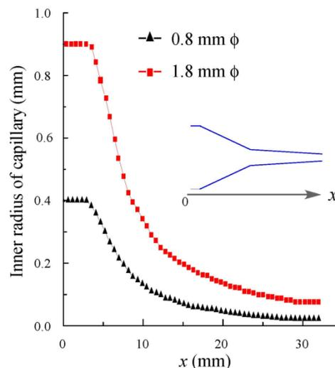
**Figure 6.** Comparison of the inner radius of the capillary between the 1.8 mm and 0.8 mm inlet diameters.
