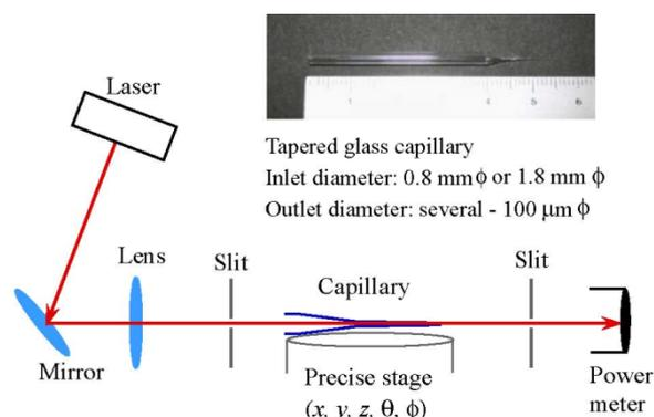
Figure 1. Experimental setup for transmittance measurements.
