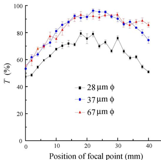
**Figure 3.** Dependence of transmittance on the position of the focal point for the 1.8 mm inlet diameter at 488 nm. The origin of the  $x$  axis is set at the position of the capillary outlet.
