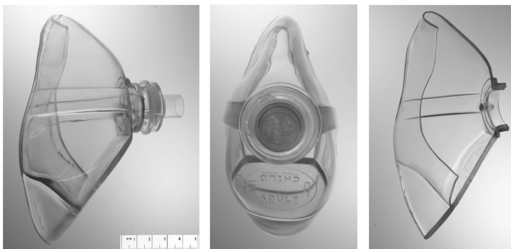
Figure 1. The Test BVM consisted of a pliable facemask and a rigid non-rebreathing valve. All residual bioburden analysis methods were completed on masks that were cut in half after removal of the valve.
