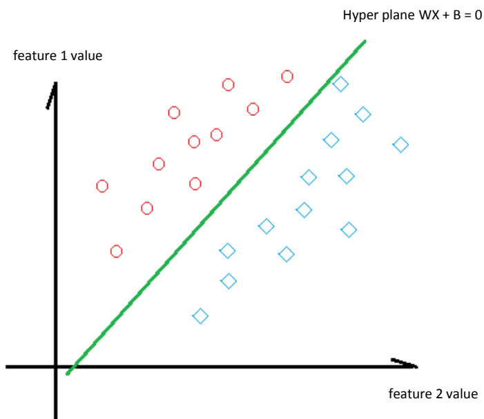
Figure 1. The principle of classification using SVM with two features.
