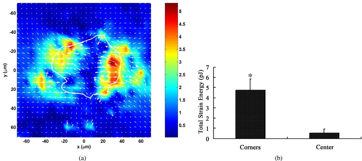
**Figure 3.** (a) Distribution of average traction (mean,  $n = 13$ ). Color of the map denote the magnitude and arrows do the magnitude and direction of the tractions; (b) Results of relative traction forces (pJ) in cell center and corners: the relative traction forces in cell corners were nearly 10-fold more than cell center.
