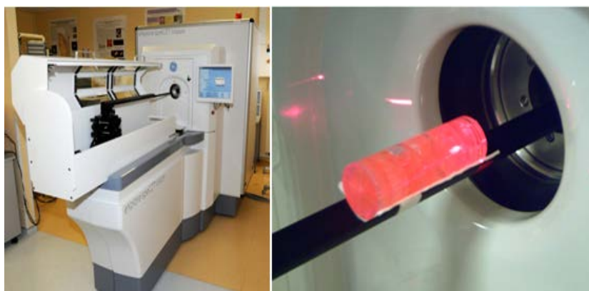
Figure 1. Phantom placed in the tunnel of the speCZT eXplore CT 120 machine.
