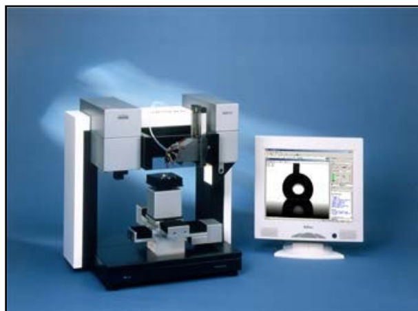
Figure 3. The goniometer employed by us (Tropfenkontur-Analyse system DSA100).
