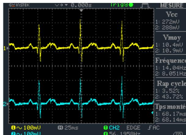
**Figure 13.** The upper signal is the retrieved (decrypted) ECG signal for  $R_{11} = 1 \text{ K}\Omega$  and  $C_3 = 10 \mu\text{F}$  while the lower one is the original ECG.
