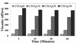
**Figure 3.** Viscosity measurement of the hydrogel depending on HAp concentration (p < 0.05; n = 3).
