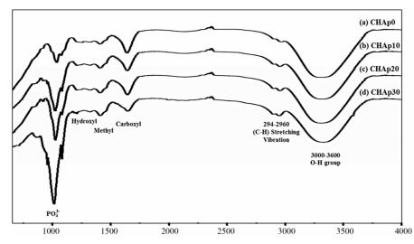
Figure 2. FT-IR spectra of the fabricated CMC hydrogels modified with varying concentrations of HAp.
