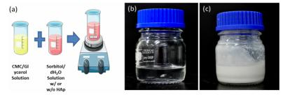
**Figure 1.** Experimental procedure in the preparation of the hydrogel (a) and photograph of CMC hydrogel without HAp (b) and CMC hydrogel with Hap (c).
