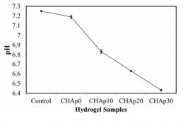
**Figure 4.** Analysis of the pH value of the hydrogel depending on Hap concentration (p < 0.05; n = 5).
