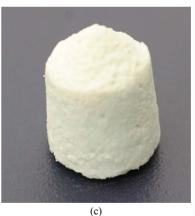
**Figure 2.** (a) Bentonite clay; (b) Sodium metasilicate and (c) bioceramic monolith with Bioglass<sup>®</sup> 45S5 composition.
