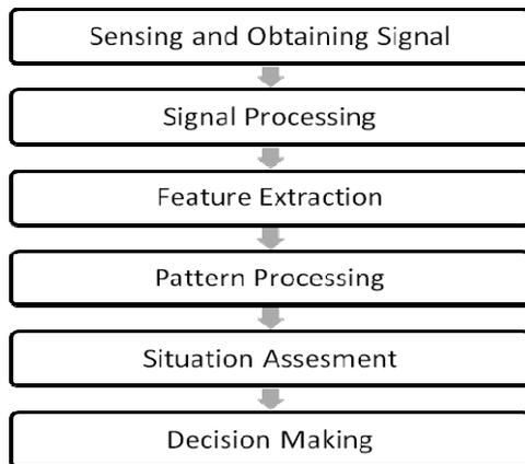
**Figure 1.** The “waterfall model” of information fusion.
