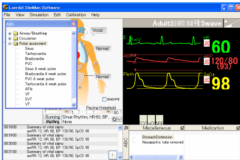
Figure 2. A control window on the main window of HPS. A list of training pulses is displayed in the control window. The ECG, arterial pulse and saturation of oxygen are sequentially drawn in a monitor panel on the main window. The two windows are only shown in operator's PC. The display is hidden to participants in training.
