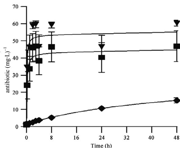
**Figure 2.** Elution of antibiotic from gentamicin sulphate (■) S ( $n = 8$ ), gentamicin palmitate (◆) ( $n = 5$ ) and vancomycin (▼) coated K-wires. K-wires were immersed in PBS, and 500  $\mu$ l aliquots taken over 48 hours. Data is presented as the mean concentration of antibiotic in the gentamicin sulphate ( $n = 8$ ) and gentamicin palmitate ( $n = 5$ ) and vancomycin ( $n = 8$ ) solutions. Error bars represent the SEM.
