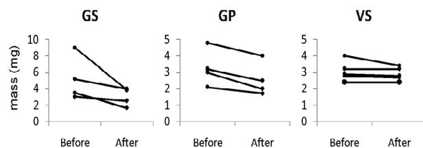
**Figure 1.** Loss of coating mass after abrasion testing. Coated K-wires were weighed prior to, and after being passed through a 1.8 mm bore hole in bovine cortical bone. Data points representing individual K-wires prior to and after passing through the bone are connected by the lines.
