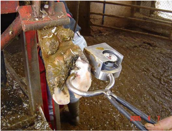
Figure 2. An instrumented hoof tester is used to assess the force that elicits hoof pain reaction. Sound cattle can sustain 75 Kg with no reaction. The ratio of the force eliciting hoof pain reaction and 75 Kg is proposed as a hoof pain index.
