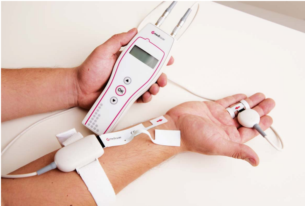
Figure 1. The new device (Mediracer®, Mediracer International, Oulu, Finland) uses two self-adhesive, disposable hydrogel coated electrodes. One is a stimulating electrode that wraps around the finger being tested and the second is a recording electrode that is placed over the wrist.
