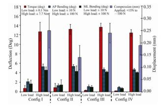
**Figure 7.** Construct stability properties for each screw configuration of Part II.
