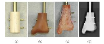
**Figure 3.** Samples of the experiment test specimens. (a) Part I test specimen (PVC), (b) Part II test specimen (composite analogue bone), (c) Part III test specimen (Cadaver), and (d) Radiograph of Part III test specimen.
