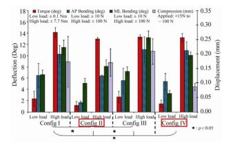
Figure 6. Construct stability properties for each screw configuration of Part I.
