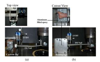
**Figure 5.** Bending experimental setup. (a) Part I experimental setup, (b) Parts II and III experimental setup.
