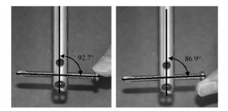
Figure 9. Screw movement within the interlocking screw-hole.
