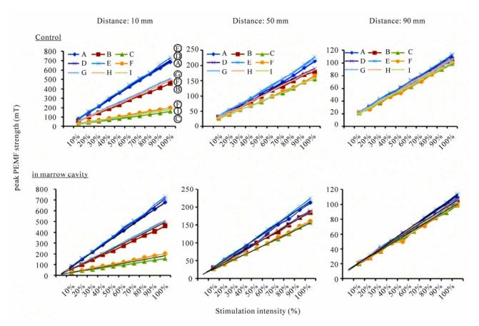
**Figure 2.** Relationships between peak PEMF strength and stimulation intensities in marrow cavity and control conditions. Note the 3 types of geometric difference in PEMF strength correlating with stimulation intensity and distance, with the highest values for positions A-D-E, middle values for B-G-H and lowest values for C-F-I. Positions A-I are the same as in **Figure 1**.
