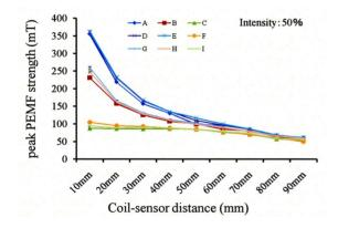
**Figure 3.** Relationships between peak PEMF strength and coilsensor distance at 50% stimulation intensity and at 9 positions (A-I).
