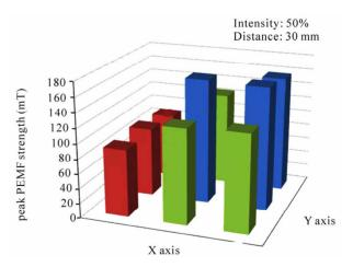
**Figure 4.** Relationships between peak PEMF strength and horizontal positions (A-I) at 50% stimulation intensity and 30 mm coil-sensor distance.
