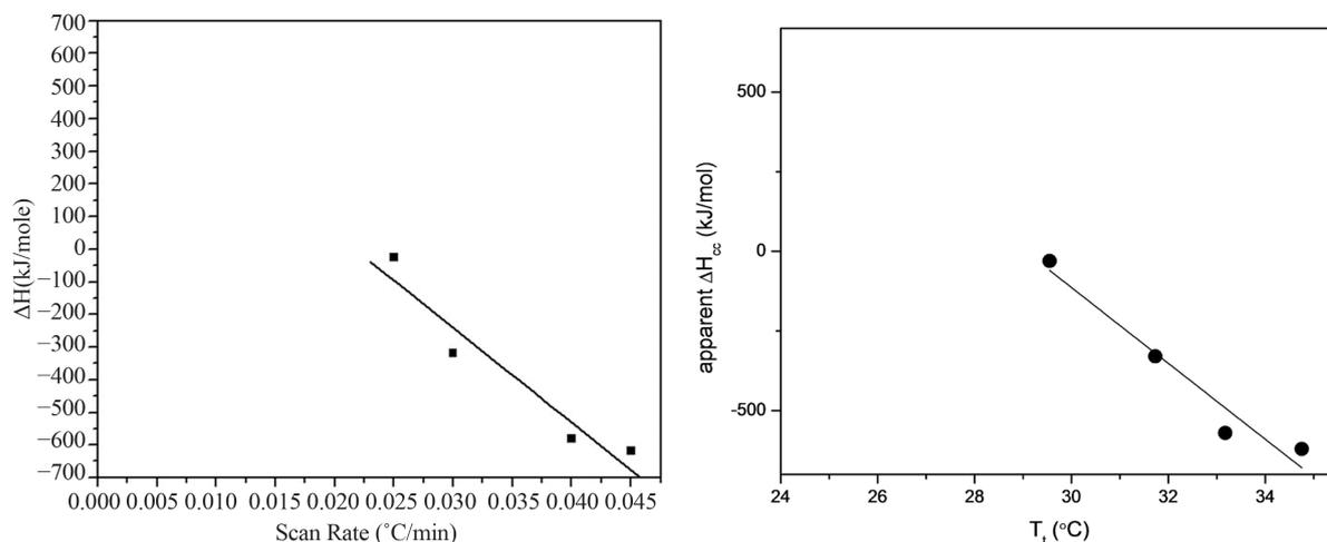
**Figure 6.** Methods for the evaluation of  $\Delta H_{pc}$ . A plot of the observed enthalpy changes vs. scan rate yields a value of  $6.3 \times 10^2 \pm 2.1 \times 10^2 \text{ kJ}\cdot\text{mol}^{-1}$  (left) and vs. apparent temperature of the transition yields  $6.0 \times 10^2 \pm 1.1 \times 10^2 \text{ kJ}\cdot\text{mol}^{-1}$ .
