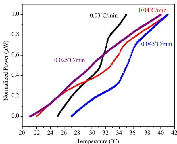
**Figure 2.** Normalized (with respect to instrument power output), baseline-corrected ssrDSC measurements of  $2.0 \text{ mg}\cdot\text{mL}^{-1}$  samples of TLX in 150 mM sodium phosphate buffer (pH = 7.0,  $p = 1.00 \text{ atm}$ ). Scan rates are indicated.
