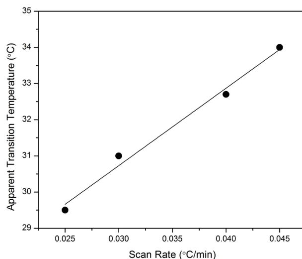
**Figure 3.** Apparent transition temperatures of the exothermic DSC transitions at 1.0 atm as function of instrument scan rate. Extrapolation to zero scan rate yields  $24.3^\circ\text{C} \pm 0.6^\circ\text{C}$  as the equilibrium transition temperature.
