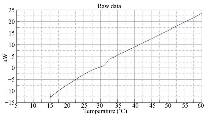
**Figure 1.** Screen capture of data obtained in a ssrDSC run of a 2.0 mg/mL sample of TLX in 150 mM sodium phosphate buffer (pH = 7.0) and at total applied pressure of 1.0 atm. Scan rate is 0.030 K·min<sup>-1</sup>. Run is not baseline corrected.
