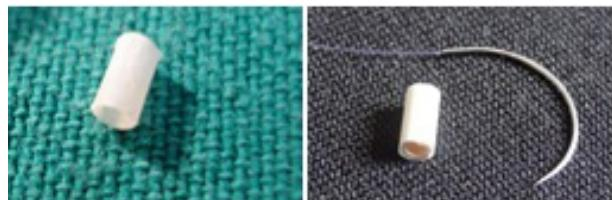
**Figure 1.** SCB tube on the left and polyurethane tube on the right.
