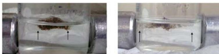
**Figure 11.** CMC-NP hydrogel between two opposing permanent magnets.
