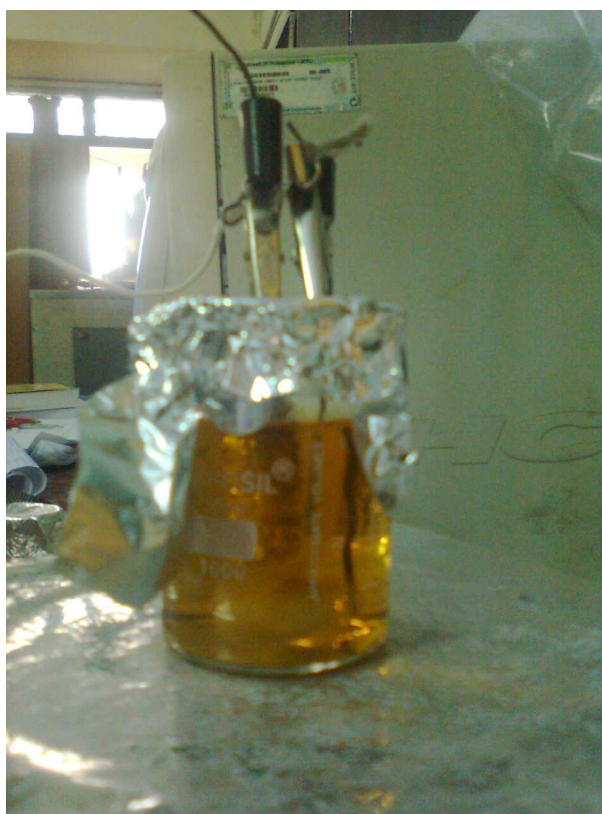
Figure 2. Synthesized colloidal solution of silver nanoparticles.
