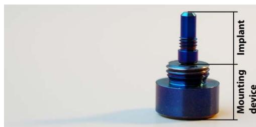
**Figure 1.** Photograph of implant where the cylindrical pin constitutes the actual sample, the screw at the top was used to fixate the implant in the cortical bone.
