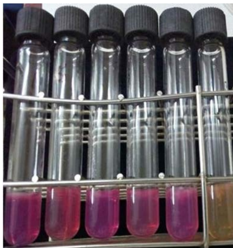
Figure 4. Urease test of some of the isolated Actinomycete showing positive urease test. The last one is a negative control.
