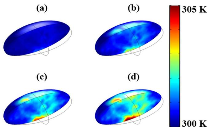
**Figure 2.** Temperature distribution of the bio-organism at different times: (a) 10 s, (b) 30 s, (c) 45 s, (d) 60 s.
