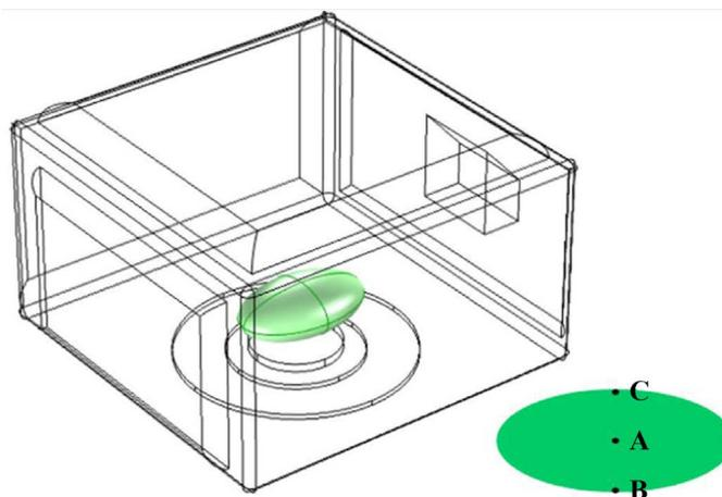
**Figure 1.** The bio-organism is located inside a metal box under the illumination of microwave. Three points located at the central plane of the bio-organism (shown in the lower right inset) are chosen to monitor the temperature and fraction of damage. (C point is center point of the upper surface, B point is center point of the surface below. A point is the central of whole bio-organism.)
