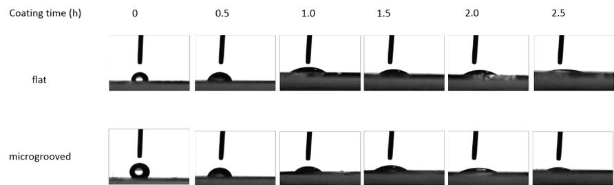
**Figure 1.** The water contact angle of PDMS substrates coated with gelatin for different time. The water contact angle of both flat and microgrooved surface of PDMS substrates before and after coating with gelatin. Coating time was optimized from 0.5 to 2.5 h.
