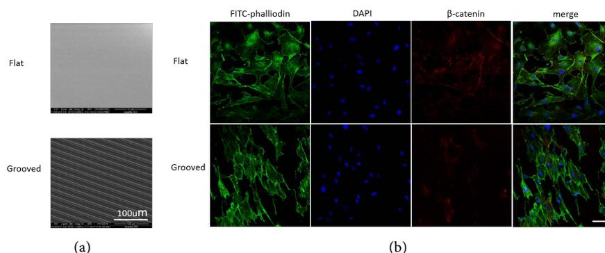
**Figure 2.** HUVEC morphology on different PDMS substrates. (a) Scanning electron micrograph (SEM) images of PDMS substrates with flat or microgrooved surface. The image of the microgrooved PDMS substrates with a 10 μm parallel grooves width and 3 μm in depth; (b) The confocal image of HUVECs cultured on flat and grooved PDMS substrates. Cells were stained with phalloidin (green), DAPI (blue), and anti-β-catenin antibody (red). Scale bar, 75 μm.
