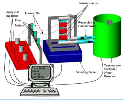
Figure 1. Sketch of the experimental setup.
