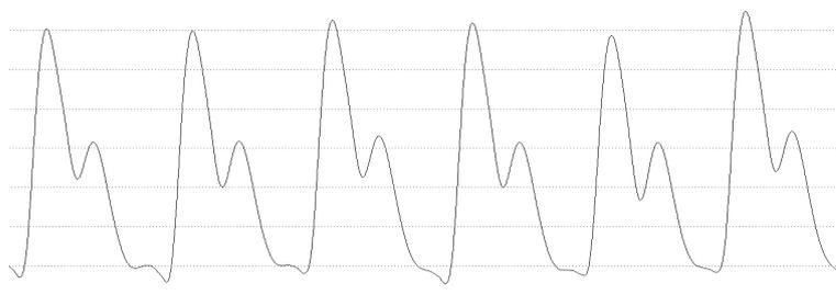
**Figure 3.** The PPG signals after removing baseline drift and smoothing.
