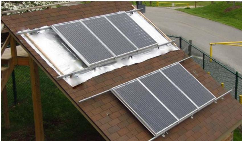
**Figure 10.** Photo of Trial 6. Upper array silver roof paint flush 3 modules, lower array shingles flush 3 modules. (Refer to [Table 1](#) for details)
