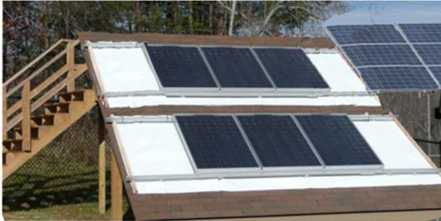
**Figure 8.** Photo of Trial 4. Upper array white TIOCOAT™ flush 3 modules, lower array white TIOCOAT™ flush 3 modules. (Refer to [Table 1](#) for details).
