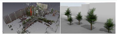
Figure 1. Co-registered TLS point clouds, and the tree model used in rendering. The feature (d) marked with a red line is 23.2 m high.
