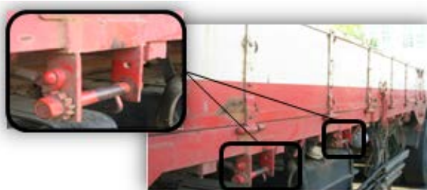
Figure 2. Fixing blocks welded to a truck [6].
