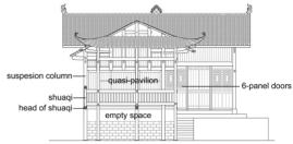
Figure 5. Façade map of the stilted building drawing by Kui Zhao, 2013.
