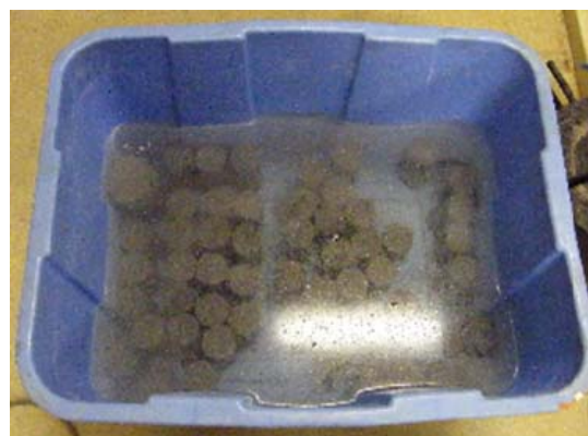
Figure 5. Curing of shell husk concrete.
