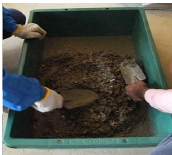
Figure 3. Dry-mixing of shell husks with sand-cement.
