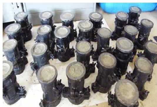
Figure 4. Casting of shell husk concrete.
