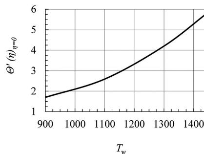
**Figure 6.** Dependence of the first derivative of the self-similar function on the temperature on the wall  $T_w$  ( $^\circ\text{C}$ ):  $T_\infty = 1450^\circ\text{C}$ ;  $Pr_\infty = 5180$ .
