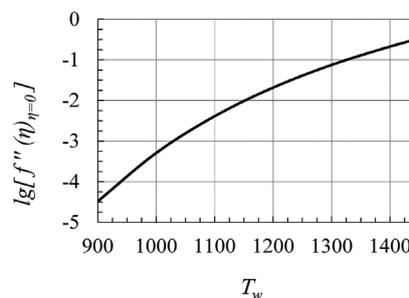
**Figure 3.** Dependence of the second derivative of the self-similar function on the wall temperature  $T_w$  ( $^\circ\text{C}$ ):  $T_\infty = 1450^\circ\text{C}$ ;  $Pr_\infty = 5180$ .
