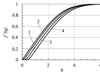
**Figure 2.** Distribution of velocity profiles in the boundary layer at: 1—Blasius solution; 2— $T_w = 1300^\circ\text{C}$ ; 3— $T_w = 1100^\circ\text{C}$ ; 4— $T_w = 900^\circ\text{C}$ ;  $T_\infty = 1450^\circ\text{C}$ ;  $Pr_\infty = 5180$ .
