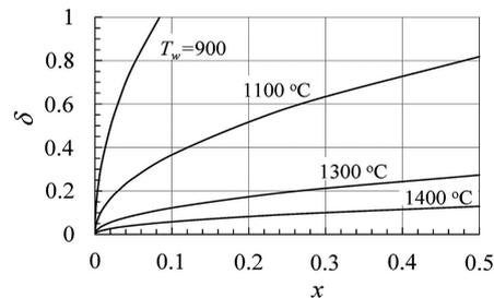
**Figure 5.** Dependence of the thickness of the protective layer  $\delta$  (m) on the  $x$  (m) coordinate (for different temperatures on the wall  $T_w$  ( $^\circ\text{C}$ )):  $T_\infty = 1450^\circ\text{C}$ ;  $Pr_\infty = 5180$ .
