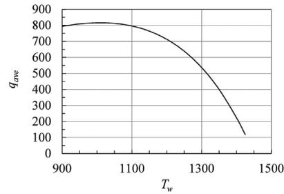
**Figure 7.** Dependence of the average heat flux density  $q_{ave}$  (W/m<sup>2</sup>) on the temperature on the wall  $T_w$  (°C):  $T_\infty = 1450^\circ\text{C}$ ;  $Pr_\infty = 5180$ .
