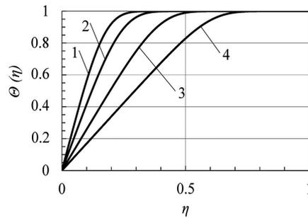
**Figure 4.** Distribution of temperature in the boundary layer at: 1—Leveque solution; 2— $T_w = 1300^\circ\text{C}$ ; 3— $T_w = 1100^\circ\text{C}$ ; 4— $T_w = 900^\circ\text{C}$ ;  $T_\infty = 1450^\circ\text{C}$ ;  $Pr_\infty = 5180$ .
