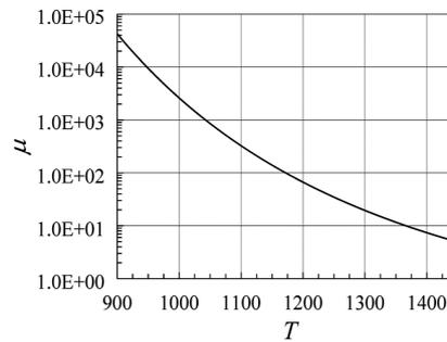
**Figure 1.** Dependence of the coefficient of dynamic viscosity on temperature for basalt from the Ivanova Dolina deposit.
