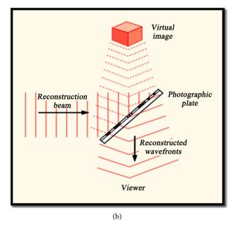
**Figure 4.** (a) Holography recording or WRITE process that generate hologram memory; (b) Activation of the source by a coherent beam or READ process that generate three dimensional image.
