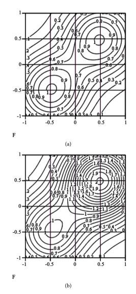
**Figure 2.** Wave superposition by different non-reactive sources. (a) Wave superposition by a non-reactive source; (b) Wave superposition by another non-reactive source.
